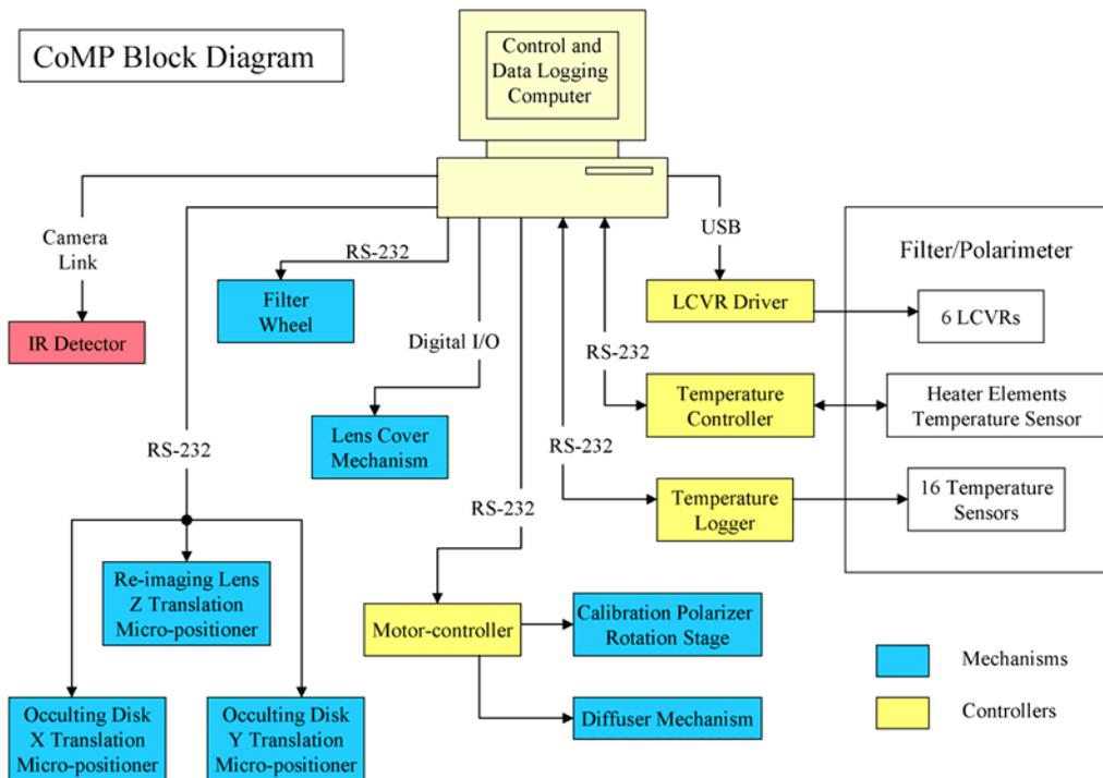
Figure 6. Block diagram of the CoMP instrument.
