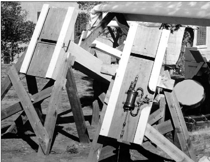
Figure 5: Campbell's moving plate spectrographs as they appeared in 1905, showing one of the gas-driven pistons that moved the plate-holder in order to obtain a continuous recording of the coronal spectrum throughout totality (courtesy: Mary Lea Shane Archives).
