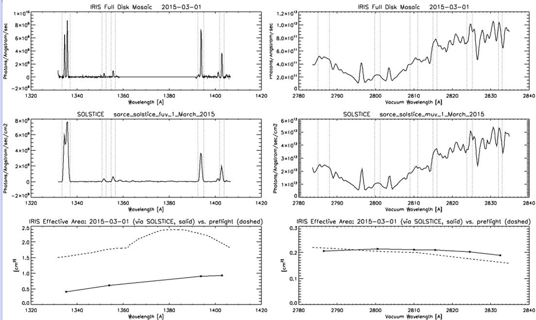
Top: Integrated IRIS FUV (left) and NUV (right) spectra of the sun from a full disk mosaic observed on 2015 March 1. Middle: SORCE/SOLSTICE spectra from the same day. Dotted vertical lines indicate the spectral windows used for cross-calibration.
